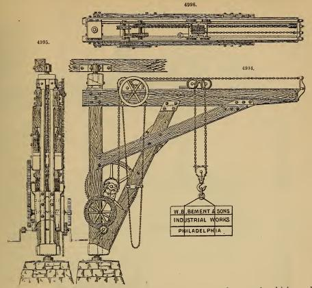
The arrangement for moving the crane longitudinally by means of spur-gearing, driving, and travelling wheels T T is similar to the plan adapted to a hand travelling crane.
